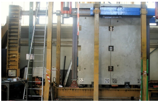
Fig. 17. View of experimental setup for the two-panel sub-assembly tests.
